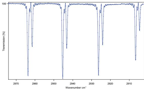
With its high resolution, the ALPHA is ideal for gas analysis. In the FT-IR spectrum of the HCl the ro-vibrational lines are split due to the chlorine 35 and chlorine 37 natural isotopic ratio of 3:1.
