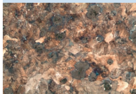
Cast iron with spherulites, etched
