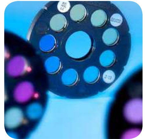
Test disc with colour-stable glass standards
