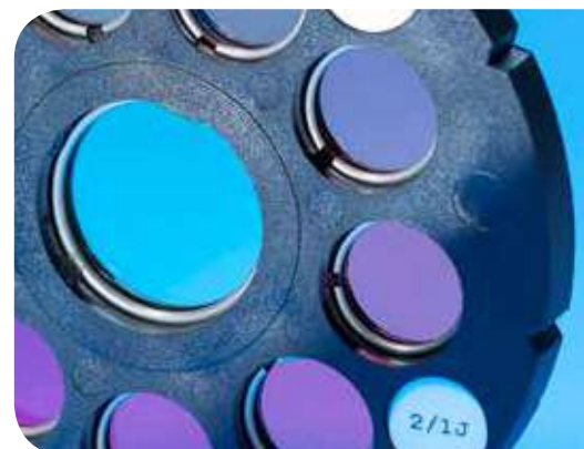
Test disc with colour-stable glass standards
