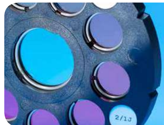
Test disc with colour-stable glass standards
