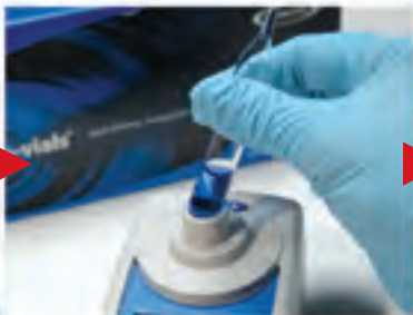
Set Reagent Blank Value using unsnapped ampoule
