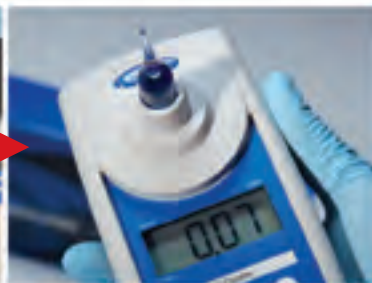
Obtain Test Results by inserting the snapped ampoule in the instrument's sample cell
