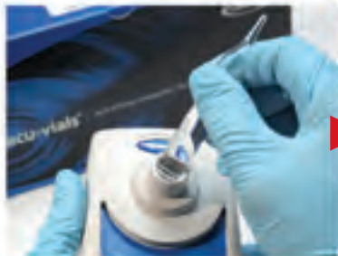
Set Instrument to Zero using the zero ampoule
