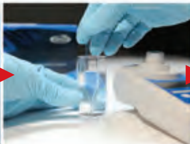
Snap the Ampoule by placing the tip at the bottom of the sample cup
