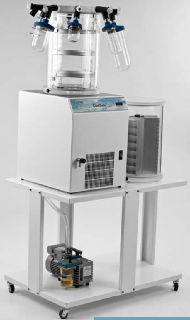
Chamber CC300-8V with shelves and manifold combined.
