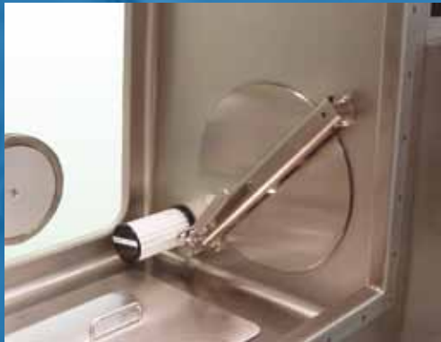
Transfer chamber door with wash tank and filter
