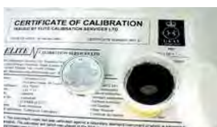
111 1056 -> SAL-T/C 11% RH 111 1057 -> SAL-T/C 33% RH 260 0190 -> SAL-T/C 58% RH 111 1063 -> SAL-T/C 75% RH 260 0276 -> SAL-T/C 84% RH 111 1065 -> SAL-T/C 90% RH 111 9981 -> SAL-T/C 97% RH
