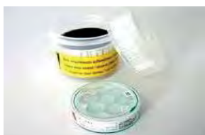
111 0930 -> SAL-T 11% RH 111 0932 -> SAL-T 33% RH 260 0189 -> SAL-T 58% RH 111 0936 -> SAL-T 75% RH 111 9886 -> SAL-T 84% RH 111 0938 -> SAL-T 90% RH 111 9887 -> SAL-T 97% RH
